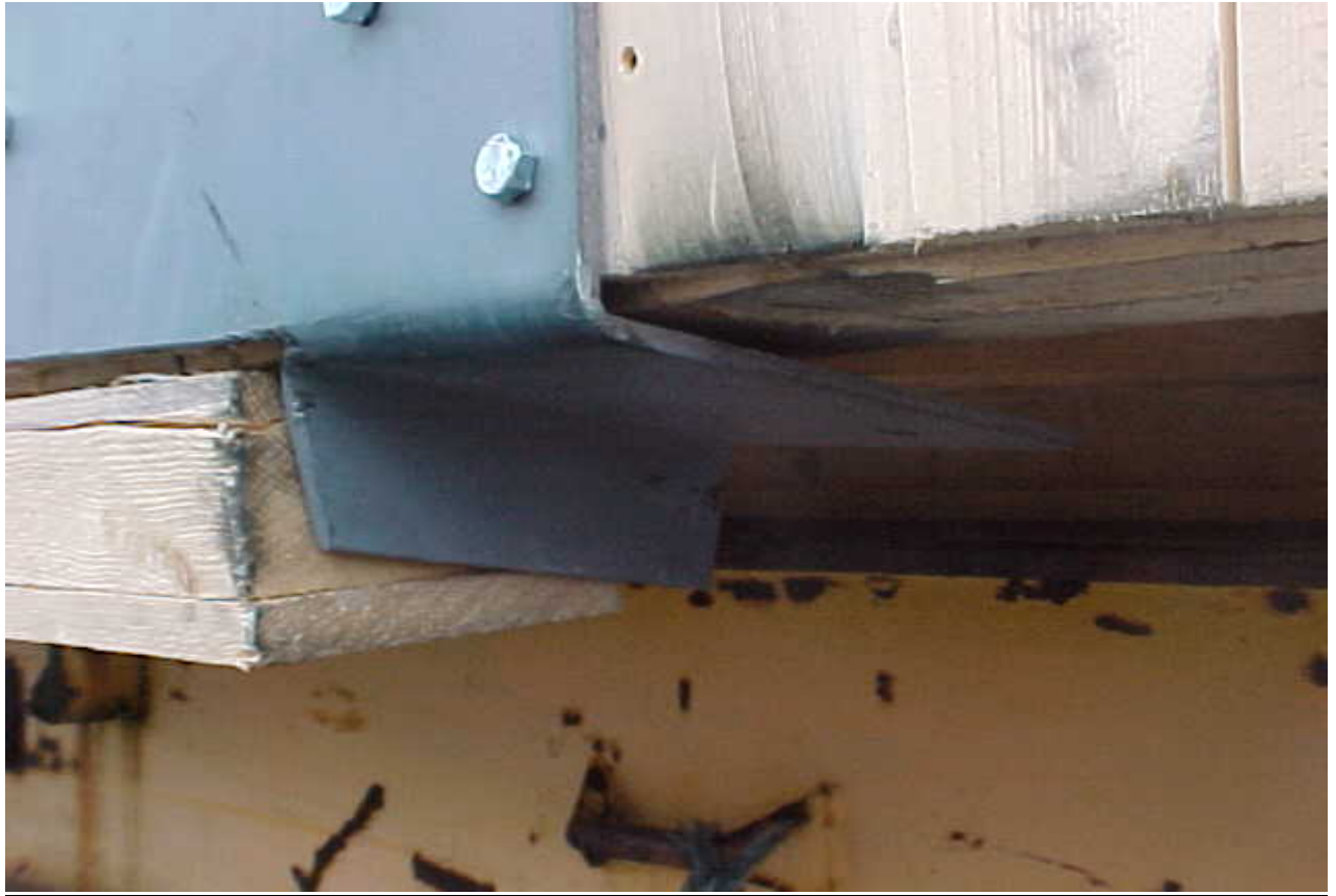
PREVIOUS MINOR DAMAGE TO SHOE PROTECTIVE AT SLING POSITION
