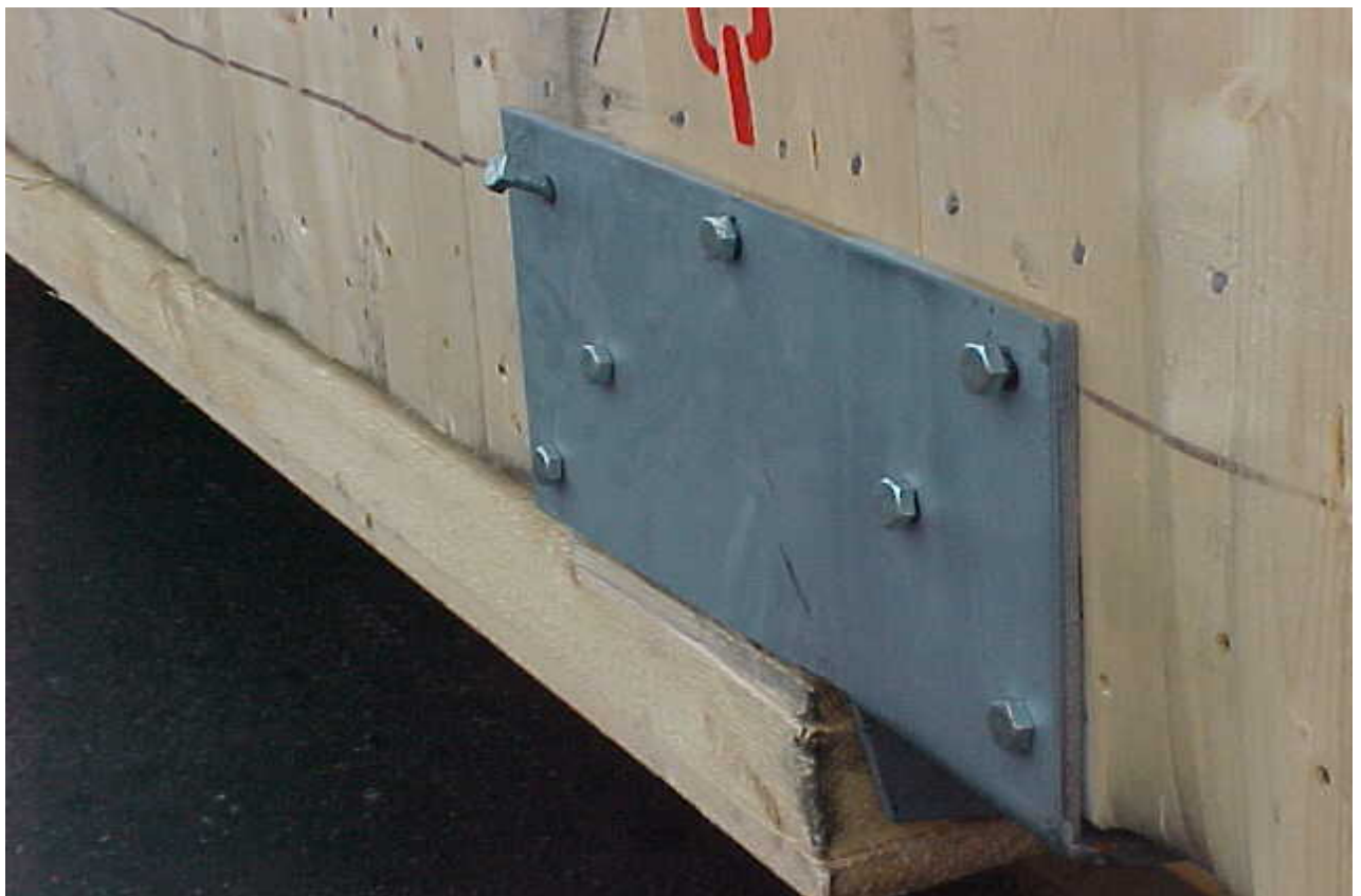
PREVIOUS MINOR DAMAGE TO SHOE PROTECTIVE AT SLING POSITION
